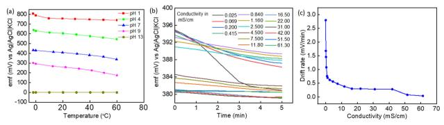
Fig. 6 (a) Influence of temperature on the emf response in various pH buffers, (b) changes of emf in the solutions with different solution conductivity, (c) influence of the solution conductivity on the drift rate of the fabricated pH sensors.
