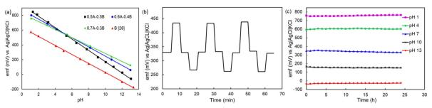
Fig. 5 (a) Comparison of the emf *versus* pH plots for the  $Co_2O_3$  (A)-RuO<sub>2</sub> (B) electrodes with 50, 60 and 70 mol%  $Co_2O_3$  (this work) and RuO<sub>2</sub> (B) electrodes (previous work.<sup>28</sup> (b) hysteresis effect for 3 cycles of 7  $\rightarrow$  4  $\rightarrow$  7  $\rightarrow$  10  $\rightarrow$  7 loop and (c) stability of the emf response of 50 mol%  $Co_2O_3$ -50 mol%  $RuO_2$  electrodes in pH buffers for 24 h.
