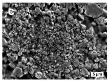
Fig. 4 SEM micrographs of samples sintered under different conditions: (a) flash-sintered sample from micropowder at 150 V cm<sup>-1</sup> and 15 mA mm<sup>-2</sup>; (b) conventionally-sintered sample from nanopowder; (c) flash-sintered sample from nanopowder at 150 V cm<sup>-1</sup> and 15 mA mm<sup>-2</sup>.
