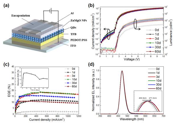
Fig. 1 (a) Device structure, (b) J-V-L, (c) EQE-J, inset is the EQE<sub>max</sub> changes over time. (d) EL spectra of blue QLEDs with encapsulation stored for different days in a nitrogen-filled glovebox.
