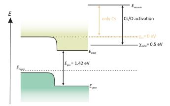
Fig. 8 Schematic drawing of the band structure of p-GaAs, activated in a YoYo process with Cs and O<sub>2</sub>.
