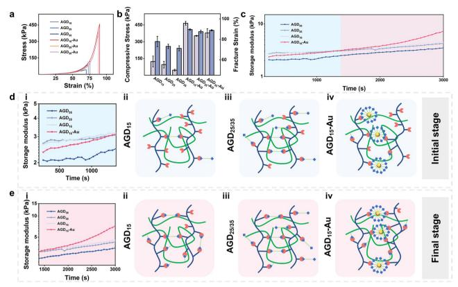
Fig. 3 (a) Compressive curves, (b) stress and fracture strain of AGD/AGD-Au hydrogels (AGD<sub>15</sub>/AGD<sub>25</sub>/AGD<sub>35</sub>/AGD<sub>15</sub>-Au/AGD<sub>25</sub>-Au/AGD<sub>25</sub>-Au), (c) the storage modulus of the prepare hydrogel vs. the time ( $AGD_{15}$ -Au/ $AGD_{25}$ -Au/ $AGD_{35}$ -Au), and (d) rheological property at the initial and final stages and (ii)-(iv) gelation mechanism of AGD-Au hydrogels
