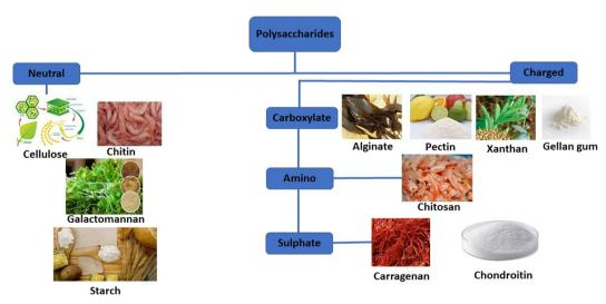
Fig. 4 The categorization of common polysaccharides that are widely deployed in the drug delivery field.
