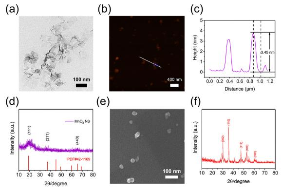
Fig. 1 Characterization of MnO<sub>2</sub> NS and CaO<sub>2</sub> NPs. (a) TEM image of MnO<sub>2</sub> NS. (b) AFM image and (c) the corresponding height image of MnO<sub>2</sub> NS dispersed on a mica substrate. (d) XRD patterns of bulk  $\delta$ -MnO<sub>2</sub> NS. (e) SEM image and (f) XRD pattern of CaO<sub>2</sub> NPs.
