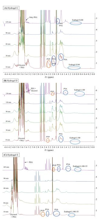
Fig. 7  $\,^{1}$ H-NMR spectra (300 MHz, BSS/D<sub>2</sub>O 90/10) obtained during the dissolution of hydrogel C (A), hydrogel D (B), and hydrogel E (C) with BSS at a constant flow rate of 110  $\mu$ L min<sup>-1</sup> at 37  $\,^{\circ}$ C. For hydrogel C (A), the spectrum was shifted by -0.24 ppm for 145 min to improve the observation of the signals. For hydrogel D (B), the spectrum was shifted 130 min by -0.24 ppm and for hydrogel E (C), the spectrum was shifted 105 min by -0.24.
