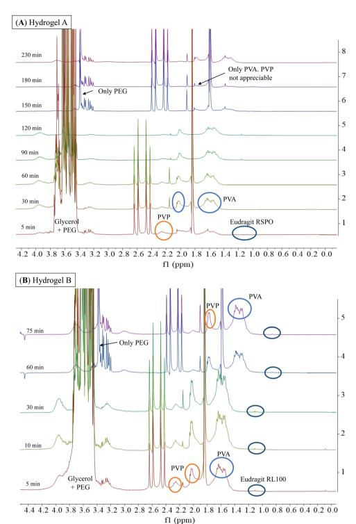
Fig. 6 <sup>1</sup>H-NMR spectra (300 MHz, BSS/D<sub>2</sub>O 90/10) were obtained during the dissolution of hydrogel A and hydrogel B with BSS at a constant flow rate of 110  $\mu$ L min<sup>-1</sup> at 37 °C. For hydrogel A, the spectra were shifted 150 min, 180 min, and 2300 min by -0.24 ppm to improve the observation of the signals. For hydrogel B, the 60 min and 75 min spectra were shifted by -0.24 ppm.
