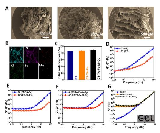
Fig. 3 (A) SEM images of CT, CT-TA-Fe, and CT-TA-Fe-MnO<sub>2</sub>. (B) Energy-dispersive spectroscopy (EDS) mapping images of CT-TA-Fe-MnO<sub>2</sub>. (C) Initial water content of hydrogels. (D)–(F) Storage modulus (G') and loss modulus (G'') of CT, CT–TA–Fe, and CT–TA–Fe–MnO<sub>2</sub> versus frequency (Hz) (G) Storage modulus of CT, CT-TA-Fe, and CT-TA-Fe-MnO<sub>2</sub>; inset shows injectable properties of CT-TA-Fe-MnO<sub>2</sub>
