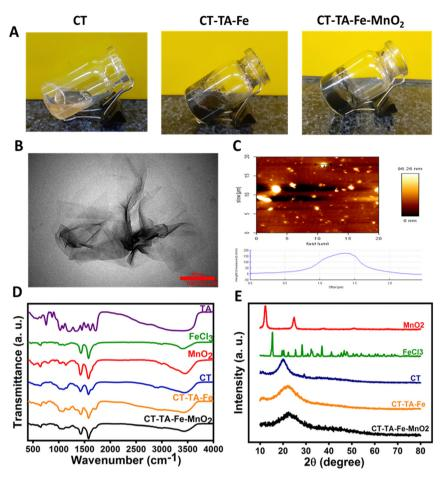
Fig. 2 (A) Photographs of CT, CT-TA-Fe, and CT-TA-Fe-MnO<sub>2</sub>. (B) TEM image of MnO<sub>2</sub> nanosheets (scale bar = 200 nm). (C) AFM image of MnO<sub>2</sub> sheets. (D) FT-IR spectra and (E) XRD pattern of CT, FeCl<sub>3</sub>, CT-TA-Fe, MnO<sub>2</sub>, and CT-TA-Fe-MnO<sub>2</sub>.
