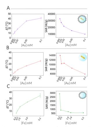
Fig. 3 Average PTH temperature increase ( $\Delta T$ , °C) and estimated SAR, using conditions of 5 min irradiation (808 nm) at 2.5 W cm<sup>-2</sup> in solution, at different concentrations of AuNR@SiO2@IONPs (A), AuNR@SiO2 (B), and  $SiO_2$ @IONPs (C). Results show mean  $\pm$  SD of triplicate measurements (error bars for SAR are within the symbols).
