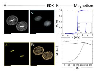
Fig. 2 (A) EDX analysis of AuNR@SiO2@IONPs, showing the elemental distribution of Au, Fe and Si. Scale bars correspond to 100 nm. (B) Hysteresis loop and ZFC/FC curves for AuNR@SiO2@IONPs. The inset in (B) shows a magnification of the central area of the curve, in which coercivity and remanence are appreciated to be negligible.
