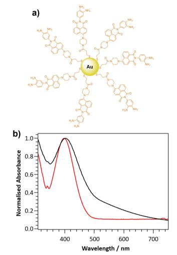
Fig. 1 (a) Schematic representation of DANPY-NO@AuNPs: AuNPs functionalised with the NO sensitive ligand DANPY-NO-ligand; and (b) normalised extinction spectrum of DANPY-NO@AuNPs (DMSO/H2O (5:2), black) and normalised UV-Vis absorption spectrum of DANPY-NO-ligand (DMSO, red).
