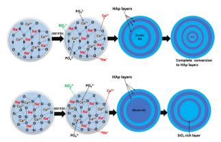
Degradation process of borate and silicate bioactive glass.
