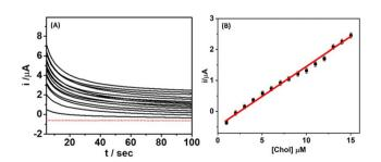
Fig. 4 (A) Chronoamperometric response of the microneedle sensor toward increasing concentrations of cholesterol (1  $\mu M$  increments) in an artificial interstitial fluid sample over the 1–15  $\mu M$  range; potential applied at +0.65 V (vs. Ag/AgCl). (B) The respective calibration plots up to 15  $\mu$ M cholesterol based on sampling the current at 100 s.
