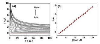
Fig. 3 (A) Chronoamperometric response of the microneedle sensor toward increasing concentrations of cholesterol (1  $\mu M$  increments) in PBS solution over a 1–20  $\mu$ M range; the potential was applied at +0.65 V (vs. Ag/AgCl). (B) The respective calibration plots for up to 20  $\mu M$  cholesterol based on sampling the current at 100 s.
