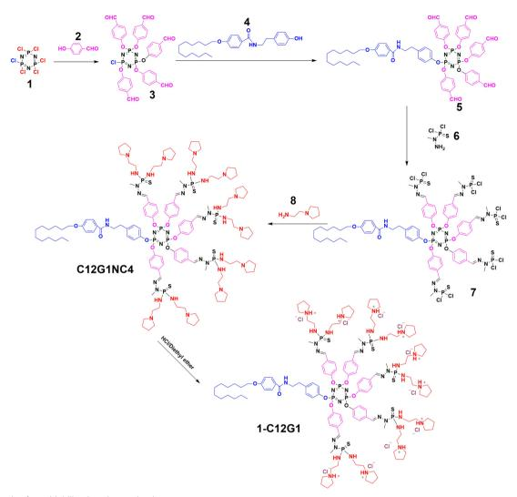
Fig. 1 Synthesis of amphiphilic phosphorus dendrons.
