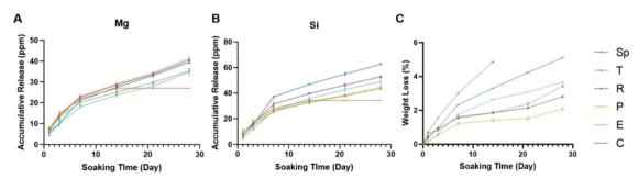
Fig. 4 Degradation profile and the weight loss of the succulent plant-like biomimetic scaffolds. (A) The accumulative release amount of Mg ions from the scaffolds in Tris-HCl solution at different time points. (B) The accumulative release amount of Si ions from the scaffolds in Tris-HCl solution at different time points. (C) The weight loss of the succulent plant-like biomimetic scaffolds and control scaffolds after soaking in Tris-HCl solution for different periods (n = 3).
