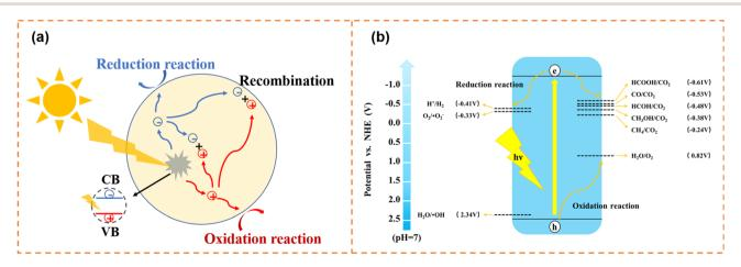
Fig. 1 (a) Schematic diagram of the photogenerated carrier transfer process. (b) Schematic illustration of thermodynamic requirements for photocatalysis.
