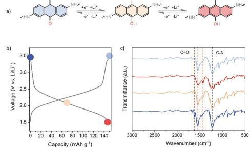
Fig. 3 (a) Electrochemical mechanism of DAAQ-TFP-COF. (b) Galvanostatic curve showing the ex situ FTIR sampling points. (c) Ex situ FTIR spectra of DAAQ electrodes in different states of charge: pristine electrode (dark blue), electrode at 0.5 SOC (yellow), electrode at 1.5 V (fully discharged, red), and electrode fully charged back to 3.5 V (light blue).
