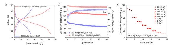
Fig. 4 (a) Galvanostatic charge/discharge curves of DAAQ-TFP-COF in 0.6 M MgTFSI<sub>2</sub> – 1.2 M MgCl<sub>2</sub> DME (red) and 0.2 M Mg(B(hfip)<sub>4</sub>)<sub>2</sub> DME (blue). (b) Evolution of discharge capacity and coulombic efficiency over 100 cycles. (c) Rate capability performance in chloride-containing electrolyte. All the experiments were conducted in Mg metal half-cells.
