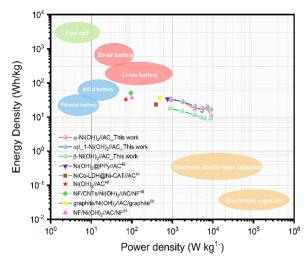
Ragone plot of Ni(OH)<sub>2</sub>//AC hybrid supercapacitors.<sup>46–51</sup>
