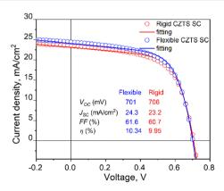
Fig. 15 J-V curves of rigid and flexible CZTS monograin layer solar cells.
