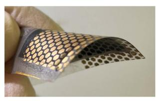
Fig. 1 Photo of a flexible CZTS monograin layer device with size of 2.5 cm  $\times$  2.5 cm.
