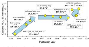
Evolution of kesterite monograin layer solar cell efficiency.
