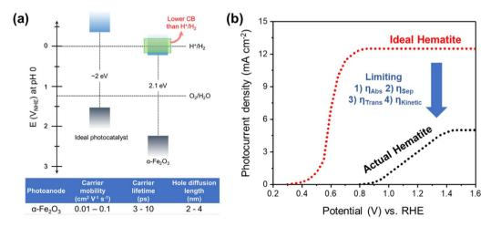
Fig. 2 (a) Band edge positions and electronic properties of hematite. (b) PEC performance of the ideal hematite photoanode and actual hematite photoanode.
