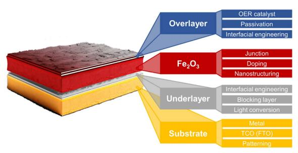
Fig. 3 Schematic illustration of various strategies for enhancing PEC efficiencies of a hematite photoanode.35-43
