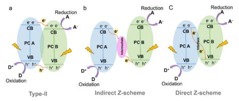
Fig. 15 Schematic illustration of the electron-transfer route in a combined system using two kinds of semiconductors with (a) type-II (b) indirect Z-scheme and (c) direct Z-scheme heterojunctions.
