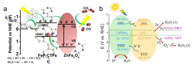
Fig. 16 The proposed charge transfer mechanisms: (a)  $ZnFe_2O_4/FeP-CTF$  for the photocatalytic  $CO_2$  reduction system. Reproduced with permission from ref. 183. Copyright 2021, Elsevier. (b)  $CsPbBr_3/CTF-2$  for photocatalytic  $H_2O_2$  production. Reproduced with permission from ref. 186. Copyright 2022, Elsevier.
