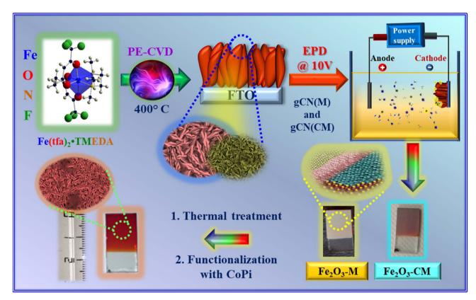
Scheme 1 Schematic illustration of the strategy used to fabricate  $Fe_2O_3$  specimens functionalized with gCN.
