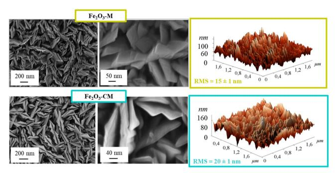
Fig. 1 Morphological characterization of Fe<sub>2</sub>O<sub>3</sub> deposits functionalized with qCN(M) (top panel) and qCN(CM) (bottom panel): FE-SEM (left) and AFM micrographs (right).
