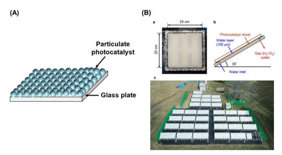
Fig. 2 (A) Schematic diagram of one-step photoexcitation based photocatalyst sheet, (B) 100 m<sup>2</sup>-scale photocatalyst panel reactor: (a) photograph of 625 cm<sup>2</sup> panel reactor unit, (b) schematic side view of panel reactor unit, and (c) top view of 100 m<sup>2</sup> solar hydrogen production system consisting of 1600 panel reactor units. Reproduced from ref. 16 with permission from Springer Nature, copyright 2021.
