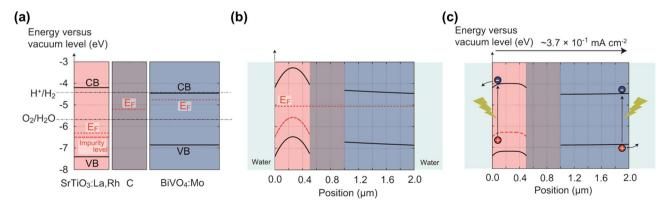
Fig. 3 Band diagrams for SrTiO<sub>3</sub>:La,Rh/C/BiVO<sub>4</sub>:Mo sheet: (a) before contact, (b) under darkness after contact, and (c) under illumination. Reproduced from ref. 28 with permission from American Chemical Society, copyright 2017.
