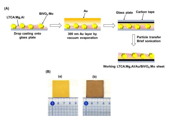
Fig. 4 (A) Schematic illustration of the preparation procedure for photocatalyst sheet composed of LTCA:Mg,Al and BiVO<sub>4</sub>:Mo. (B) Photograph of  $3 \times 3$  cm<sup>2</sup> LTCA:Mg,Al/Au/BiVO<sub>4</sub>:Mo photocatalyst sheet (a) before and (b) after particle transfer. Panel (A) was reproduced from ref. 34 with permission from Elsevier Inc., copyright 2023.
