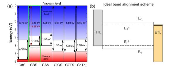
Fig. 5 (a) Vacuum-aligned band diagram between CBS and other common absorber layers. Reproduced with permission from ref. 15 Copyright 2019, the American Chemical Society. (b) Ideal band alignment scheme for CBS. HTL = hole transport layer; ETL = electron transport layer;  $E_{F^0}$  = Fermi energy level for p-type material;  $E_{F^0}$  = Fermi energy level for n-type material; EC = conduction band energy level; and EV = valence band energy level.
