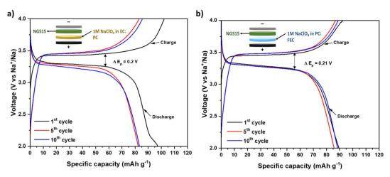
Fig. 5 Galvanostatic charge–discharge curves at 0.1C at 25 °C. (a) Na|NGS15|20  $\mu$ L of 1 M NaClO<sub>4</sub> in EC:PC|NVP and (b) Na|NGS15|20  $\mu$ L of 1 M NaClO<sub>4</sub> in PC:FEC|NVP (NGS15 was prepared *via* route 1).
