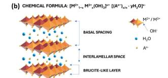
Scheme 2 Crystal structures of an (a) MXene and (b) LDH.
