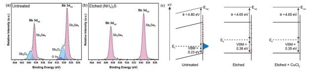
Fig. 3 Synchrotron-based XPS core level spectra of Sb 3d for (a) untreated  $Sb_2Se_3$  and (b)  $Sb_2Se_3$  etched with  $(NH_4)_2S$ . (c) Band alignment changes due to the  $Sb_2O_3$  layer (represented by the blue Gaussian) and surface states (represented by red dashes), measured by KP-FM and XPS valence band maxima (VBM). Band bending is represented as a sloping line due to the low doping (the space charge region is larger than the film thickness).
