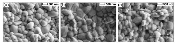
Fig. 2 SEM images for an FTO/Ti/Au/Sb<sub>2</sub>Se<sub>3</sub> sample (a) untreated, (b) etched via (NH<sub>4</sub>)<sub>2</sub>S, and (c) etched via (NH<sub>4</sub>)<sub>2</sub>S + CuCl<sub>2</sub> treatment.
