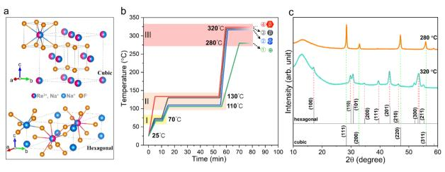
Fig. 1 (a) Schematic diagram of the crystal structure of cubic and hexagonal NaYF<sub>4</sub>. (b) Temperature profiles used for synthesizing UCNPs during the thermal decomposition process. (c) XRD patterns of NaYF<sub>4</sub> nanoparticles synthesized at growth temperatures of 280 °C and 320 °C.
