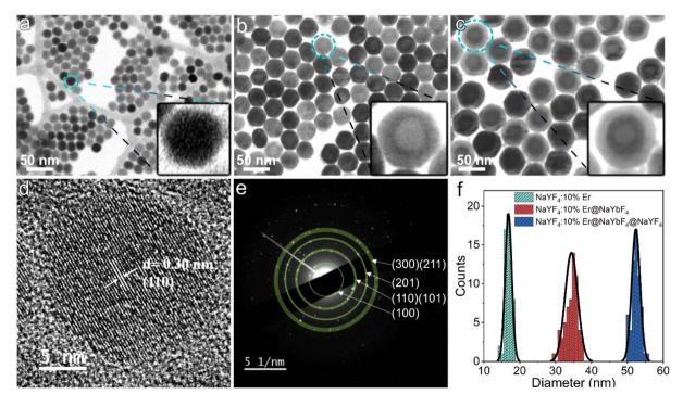
Fig. 2 SEM images of (a) NaYF<sub>4</sub>:10%Er core, (b) NaYF<sub>4</sub>:10%Er@NaYbF<sub>4</sub> core—shell, and (c) NaYF<sub>4</sub>:10%Er@NaYbF<sub>4</sub>@NaYF<sub>4</sub> core—shell—shell. (d) HRTEM image of a single NaYF<sub>4</sub>:10%Er core and (e) the corresponding SAED pattern. (f) Particle size statistics based on SEM images.
