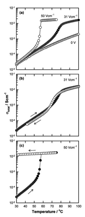
Fig. 7 Bulk conductivity of  $Bi_{0.95}Ca_{0.05}FeO_3$  against temperature without and with applied fields of 31 and 50 V cm $^{-1}$ ; reproduced from N. Maso *et al.*, *Phys. Chem. Chem. Phys.*, 2014, **16**, 19408 with permission from the PCCP owner societies.
