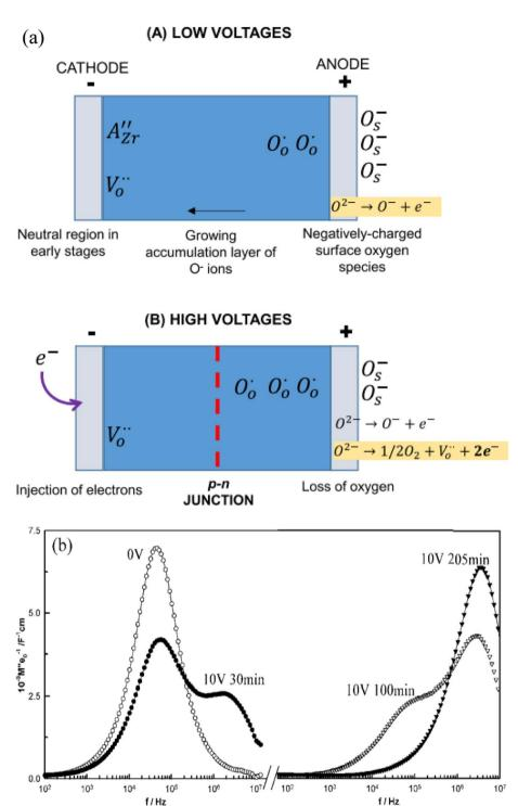
Fig. 6 (a) Model for voltage-dependent resistance at low and higher voltages; reproduced from M. Jovani et al., Sci. Rep., 2019, 9, 18538 with permission from Springer Nature; (b) M'' spectra showing evolution with time of the electrical microstructure of  $BaTi_{0.99}Mg_{0.01}O_{2.99}$  ceramic with a bias voltage of 10 V at 242 °C; reproduced from M. Prades et al., J. Mater. Chem., 2010, 20, 5335 with permission from the Royal Society of Chemistry.
