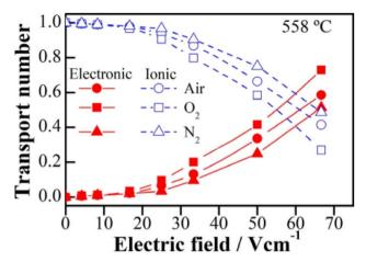
Fig. 4 Transport numbers as a function of bias voltage at 558 °C in three different atmospheres; reproduced from X. Vendrell and A. R. West, J. Am. Ceram. Soc., 2019, 102, 6100, with permission from Wiley publishing.
