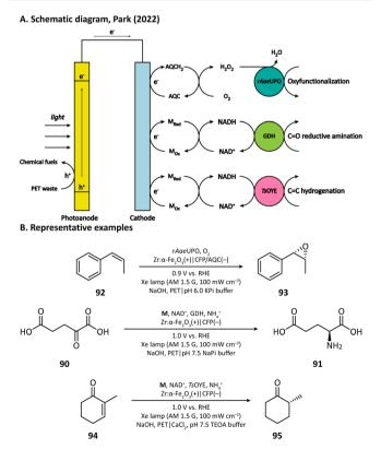
Fig. 16 PET conversion coupled with cathode-mediated biosynthesis.
