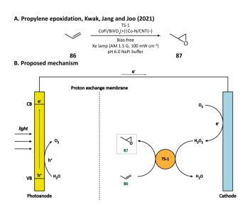
Fig. 13 Cathode-mediated in situ  $H_2O_2$  generation for propylene epoxidation.
