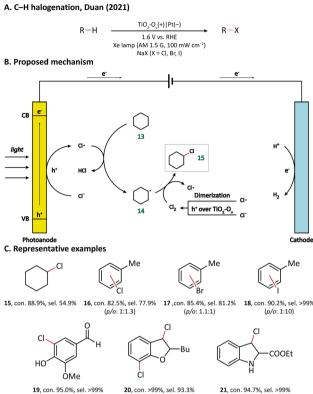
Fig. 3 Photoanode-mediated cyclohexane halogenation.
