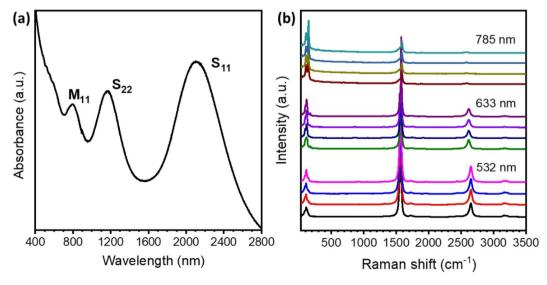
Fig. 2 Spectroscopy characterization studies of the SWCNFs. (a) The absorption spectrum of a SWCNF. (b) The Raman spectra of SWCNFs with different excitation wavelengths.
