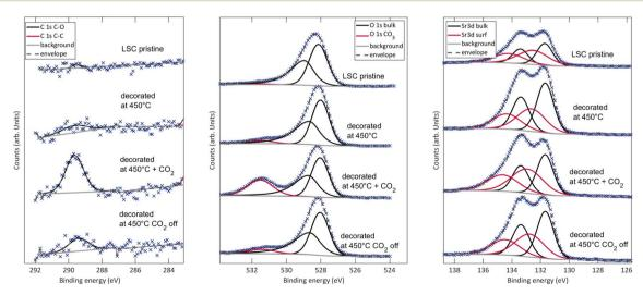
Fig. 4 XPS results for the C, O and Sr signals on pristine LSC surfaces and on low T decorated surfaces before, during and after CO₂ addition in the XPS chamber.
