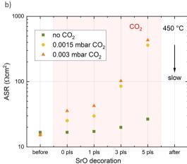
Fig. 7 Effect of *in situ* decoration from a Sr-containing target on the area specific surface exchange resistance of a dense LSC thin film at (a) high (600 °C) and (b) low (450 °C) temperatures in 0.04 mbar  $O_2$  for different amounts of additional  $CO_2$  introduced into the chamber. The arrow indicates a slow but continuous recovery of the area specific surface exchange resistance after  $CO_2$  was turned off.
