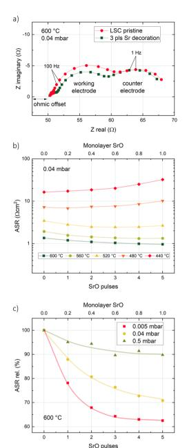
Fig. 2 (a) Exemplary impedance curves of pristine and Sr decorated LSC at 600 °C and 0.04 mbar. (b) Evolution of the area specific surface exchange resistance of a dense LSC thin film at different temperatures and 0.04 mbar  $p(O_2)$  upon in situ decoration from a Sr-containing target. (c) Evolution of the relative area specific surface exchange resistance at different partial pressures. Values are normalized to the initial resistance without Sr decoration. Lines are a guide to the eye.
