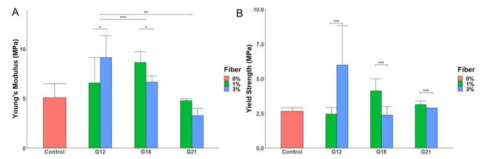
Fig. 4 (A) Young's modulus of the GIC control and GIC augmented with cellulose (1% or 3%) and left to settle for 48 h. (B) Yield strength offset from the curve by 0.2% strain of the GIC control and GIC augmented with 1% or 3% cellulose fibers. G12, G18, and G21 represent glass ionomer cement augmented with cellulose fibrils extracted using rice husk: sodium hypochlorite ratios of 1:12, 1:18, and 1:21, respectively. \*p < 0.04, \*\*p < 0.03, and \*\*\*p < 0.02.
