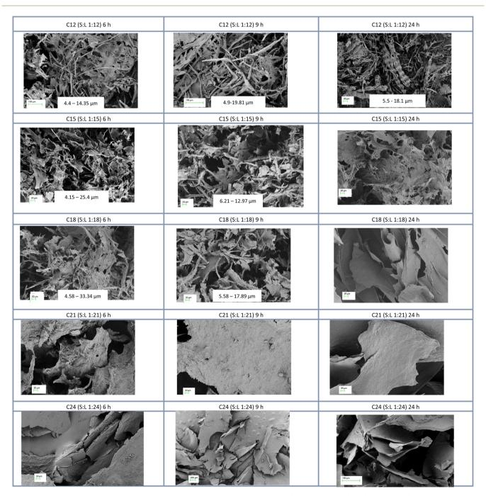
Fig. 1 SEM images of the extracted cellulose were obtained using different ratios (1:12, 1:15, 1:18, 1:21, and 1:24) of solid rice husk to hypochlorite solution and different extraction times (6, 9, and 24 h).
