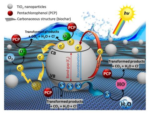
Possible reaction mechanisms of CGBT for the photocatalytic degradation.
