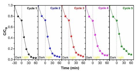
Fig. 10 The reusability potential of as-prepared CGBT nanocomposites for the photocatalytic degradation of PCP.
