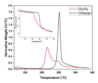
Fig. 4 TG (inset) and DTG profiles of chitosan and Chi-Py.
