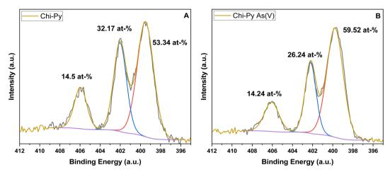
Fig. 6 The oxidation state of nitrogen via N 1s narrow scan of the pristine Chi-Py (A) and Chi-Py As(v) after (B) adsorption.
