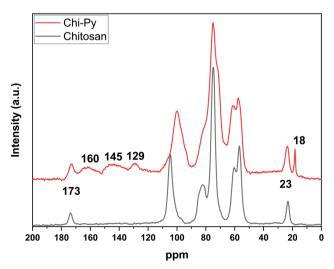
Fig. 2 <sup>13</sup>C CP-TOSS solids NMR spectra of chitosan and the pyridinium-modified chitosan.
