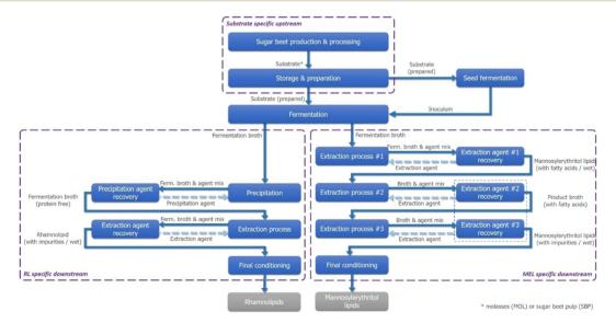
Fig. 1 Simplified aggregated flow diagram of Bio<sup>2</sup>-processes for the production of rhamnolipids (RL) and mannosylerythritol lipids (MEL); process stages represent different pooled process modules; recycling flows lead back to modules of use by the dotted line.
