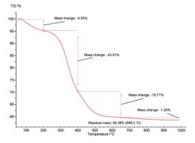
Fig. 7 TGA curve of pure sHAP (2Q: 15  $\mu$ L g<sup>-1</sup> Neutrase, 7.5  $\mu$ L g<sup>-1</sup> Lipozyme CALB L, 6 h, 40 °C) from 0 to 1000 °C.
