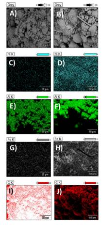
Fig. 4 SEM- EDX images. (A, C, E, G, I) Cotton post-reaction and (B, D, F, H, J) PET post-reaction. Carbon growth over the catalyst particle can be appreciated.
