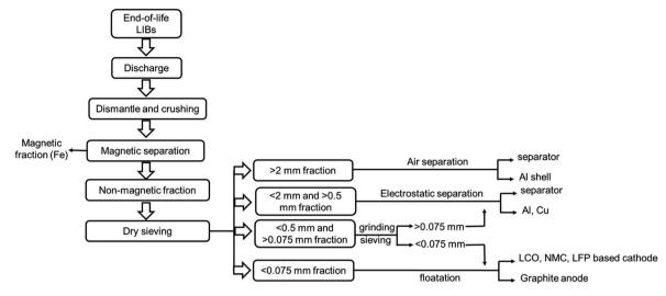
A flowchart representing the physical separation of the cell components from end-of-life LIBs based on particle size classification.
