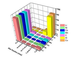
Fig. 7 Elemental distribution of the electrode components after the sieving process in different size fractions.
