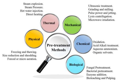
Fig. 4 Schematic representation of various pretreatment methods.
