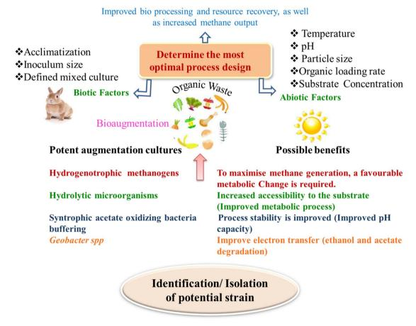
Fig. 3 Schematic representation of bioaugmentation for methane production.
