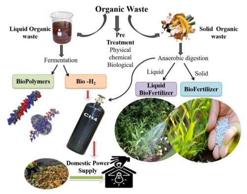
Biowaste refinery to generate high-value bioproducts and bioenergy.
