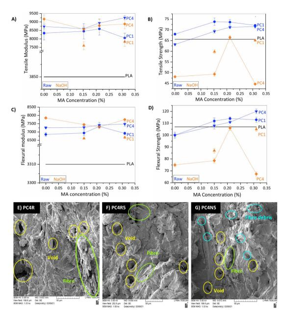
Fig. 5 (A) Tensile modulus, (B) tensile strength, (C) flexural modulus, (D) flexural strength, and SEM of the fracture surface of WPCs after tensile test. (E) PC4R; (F) PC4R5; (G) PC4N5.
