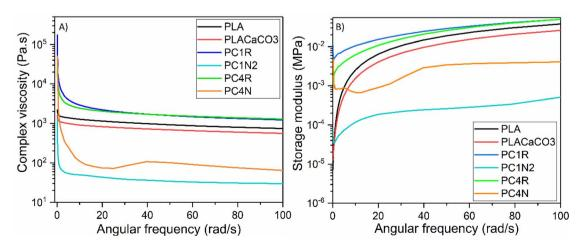
(A) Complex viscosity obtained by frequency sweep. (B) Storage modulus obtained from frequency sweep test.
