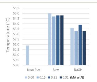
Fig. 7 HDT of PLA and WPCs reinforced with C400 fibres.
