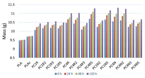
Water absorption measurements for PLA and wood plastic composites over 24, 48, and 120 hours.
