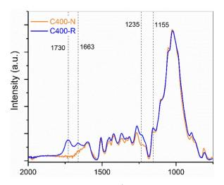
**Fig. 2** FTIR curves (2000–500 cm<sup>-1</sup>) of raw and alkalinized fibres. Absorbance at 1730 cm<sup>-1</sup> corresponds to carbonyl and aldehydes, while at 1663 cm<sup>-1</sup> to conjugated an unconjugated carbonyl bands of hemicellulose. Absorbance at 1235 and 1155 cm<sup>-1</sup> corresponds to lignin constituents.
