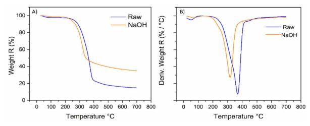
Fig. 3 (A) TGA, and (B) DTGA of raw fibres and alkaline treated fibres. Alkalinized fibres started degrading at lower temperature compared to raw fibres
