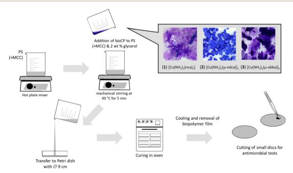
Scheme 2 Preparation of Cu-doped [PS]<sub>n</sub> and [PS-MCC]<sub>n</sub> biopolymer films.
