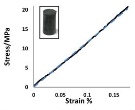
Fig. 1 Stress-strain curve for BC90 (solid line) and linear fit (dashed line). A photo of a compressive test cylinder of BC90 is shown as an inset.
