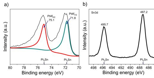
Fig. 4 XPS spectra of PtSn/VC(3), (a) Pt 4f, (b) Sn 3d.
