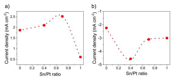
Fig. 7 Activity comparison at various Sn/Pt ratios, (a) HOR activity @ 0.2 V vs. SHE, (b) ORR activity @ 0.85 V vs. SHE. These values were determined from LSV (Fig. S10 and 11†) in 0.1 M HClO<sub>4</sub> under saturated (a) H<sub>2</sub> and (b) O<sub>2</sub>, at a scan rate of 10 mV s<sup>-1</sup> @1600 rpm. The catalyst loading was 50  $\mu$ g cm<sup>-2</sup>.
