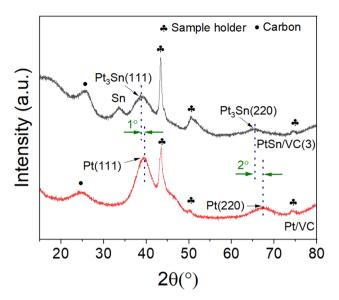
Fig. 3 XRD pattern of as-synthesized PtSn/VC(3) and Pt/VC.
