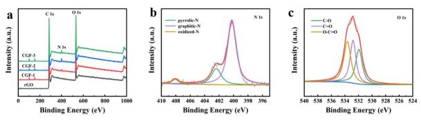
(a) XPS spectra of rGO and composite film samples; (b) N 1s spectra of CGF-2; (c) O 1s spectra of CGF-2.
