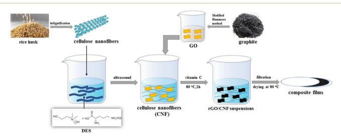
Scheme 1 Schematic illustration of the preparation of cellulose nanofibers and reduced graphene oxide composite films.
