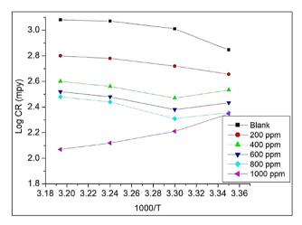
Fig. 8 Log CR (mpy) versus 1000/T for MS in Co<sub>3</sub>O<sub>4</sub>@PPy NCs.
