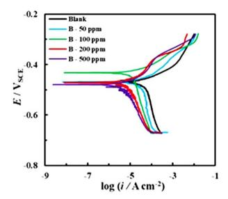
Fig. 5 Polarization curves of  $Co_3O_4$ @PPy NCs for mild steel in 0.1 M HCl at different concentrations.
