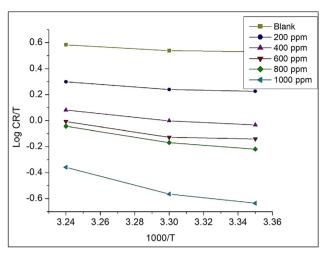
Fig. 9 Plot of log CR/T versus 1000/T for Co<sub>3</sub>O<sub>4</sub>@PPy NCs.
