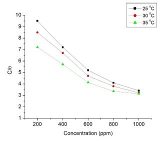
Fig. 10 Langmuir adsorption isotherm  $(C/\theta)$  versus concentration of  $Co_7O_4$ @PPy NCs at 25, 30, and 35 °C.
