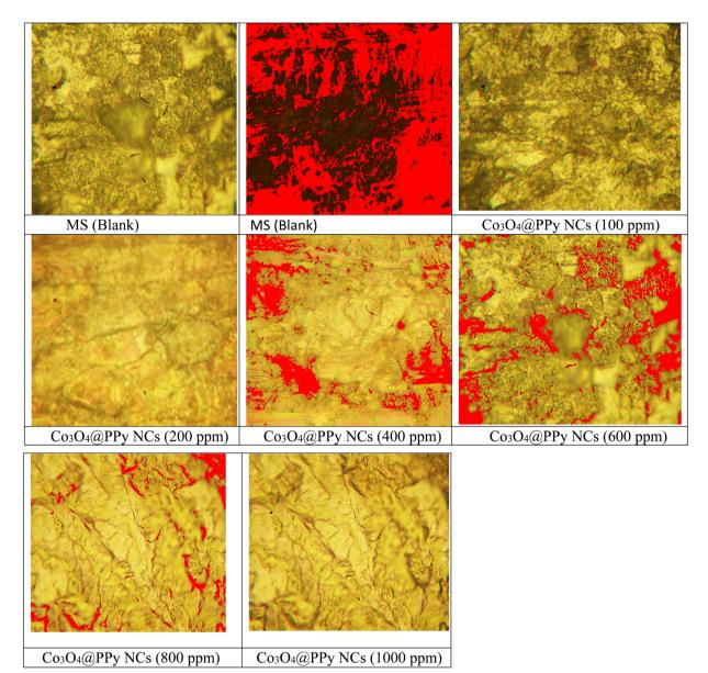
Fig. 4 Metallurgical images of blank and Co<sub>3</sub>O<sub>4</sub>@PPy NC treated MS coupons
