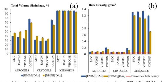
Fig. 3 Total volume shrinkage (a) and bulk density (b) of all aerogels, cryogels and xerogels made using [DBNH][OAc]/DMSO and [EMIM][OAc]/ DMSO and method 1 for cellulose coagulation. Volume and density were determined with Geopyc. The red line in (b) corresponds to a theoretical density calculated supposing no shrinkage.
