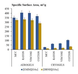
Fig. 5 Specific surface area of all aerogels and cryogels made using [DBNH][OAc]/DMSO and [EMIM][OAc]/DMSO and coagulation method 1.
