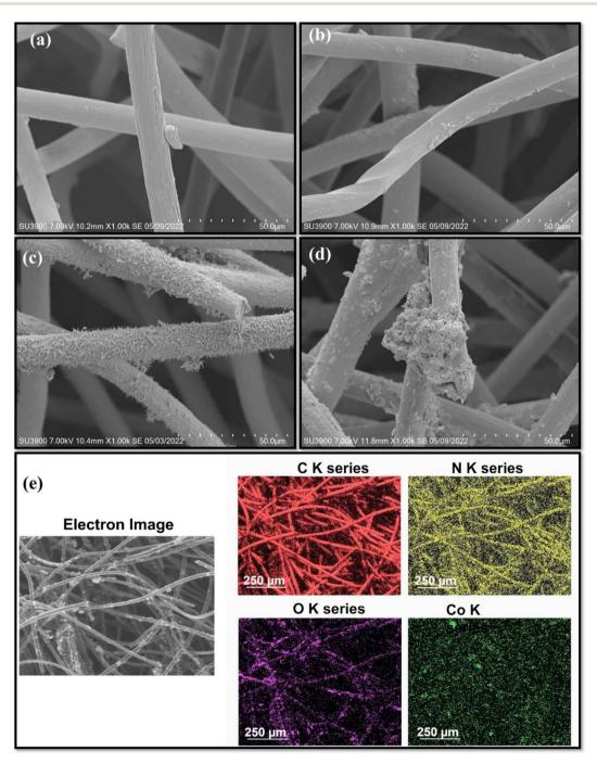
Fig. 3 SEM images of electrodes: (a) GF, (b) PANI-GF, (c) CO<sub>3</sub>O<sub>4</sub>-GF, and (d) PANI-CO<sub>3</sub>O<sub>4</sub>-GF. (e) Elemental mapping of PANI-CO<sub>3</sub>O<sub>4</sub>-GF.
