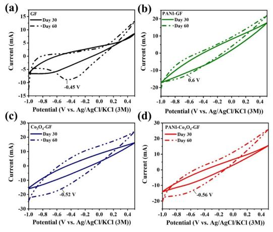
Fig. 5 Comparison of CV scans at 0.01 V s<sup>-1</sup> obtained with the anode tested in SMFCs operated for 30 and 60 days. (a) GF; (b) PANI-GF; (c)  $Co_3O_4$ -GF; (d) PANI- $Co_3O_4$ -GF. Values are averages calculated from 3 replicate anodes with a maximum standard deviation of  $\pm 6.1$  mA,  $\pm 2.4$ mA,  $\pm 4.5$  mA and  $\pm 4$  mA, respectively.
