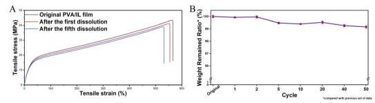
(A) Tensile stress-strain curves of the primary PVA/Br-IL film and recycled film, and (B) recycling attrition rate of the PVA/Br-IL film.
