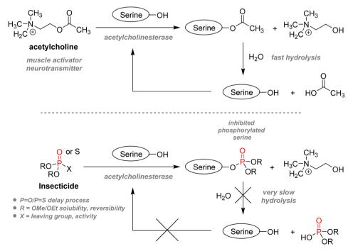
Fig. 19 Mode of action of organophosphorus acetylcholinesterase inhibitors.
